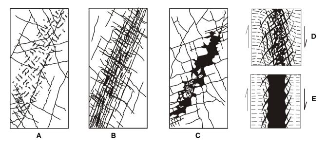
Fig. 2-6 Sketches of some types of weakness zones. A - C are from ISRM (1978) and D - E from Selmer-Olsen (1950).
