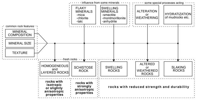
Fig. 2-3 The main variables influencing rock properties and behaviour
