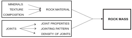
Fig. 2-1 The main features constituting a rock mass
