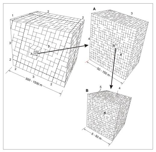
Fig. 2-8 Simplified model of various dimensions units or blocks formed by discontinuities of different size (after Pusch and Morfeldt, 1993).
