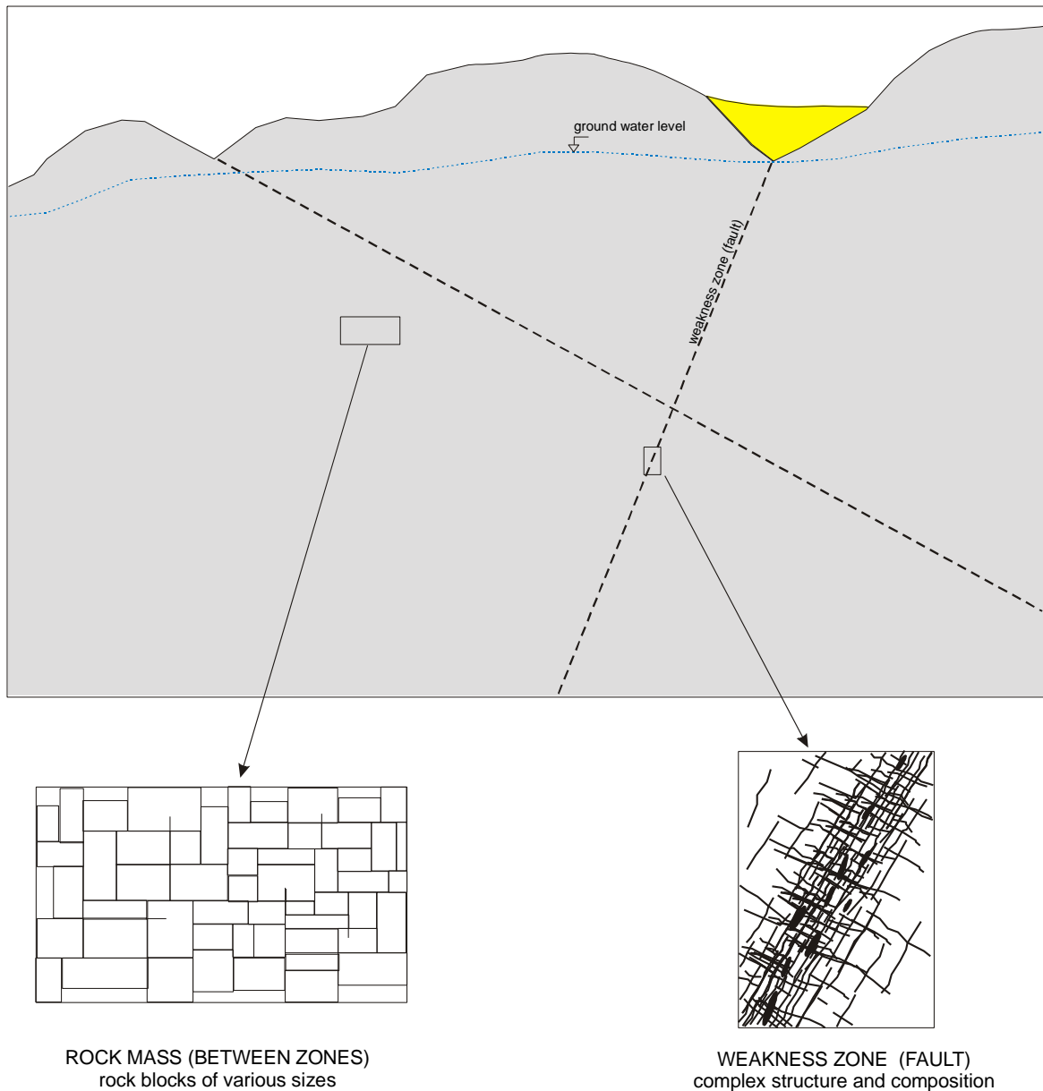
Figure 1 The two main groups of rock masses: weakness zones and rock masses between zones
