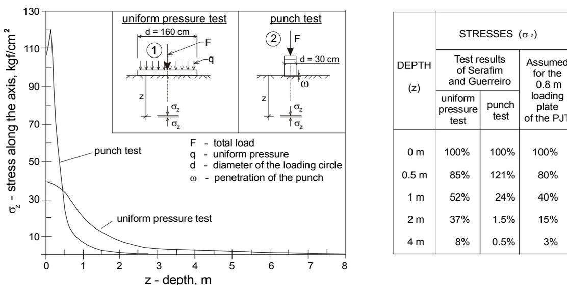
Figure 3: The distribution of stresses along beyond the loading plates ( from Serafim and Guerreiro, 1968, with modification of the table; the stresses in the right column are assumed).
