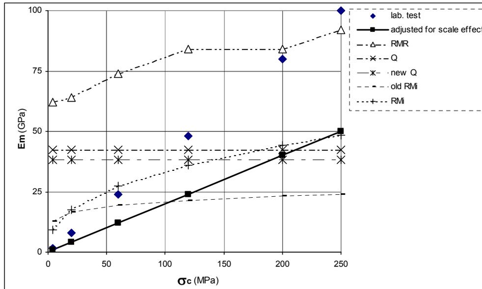
Figure 12: The deformation modulus ( $E_m$ ) in massive rock calculated from laboratory tests, RMR,  $Q$ , and RMI systems
