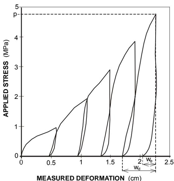
Figure 1: Typical stress versus deformation curve recorded in a deformability test of a rock mass (measured at Tala Hydropower project, Bhutan)
