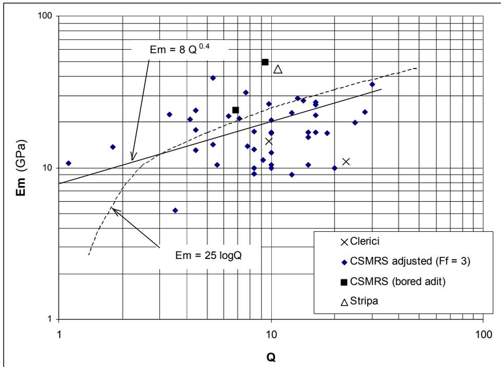
Figure 10: Connection between  $Q$  and deformation modulus ( $E_m$ ). The CSMRS (blasted) results have been adjusted with a field factor  $F_f = 3$
