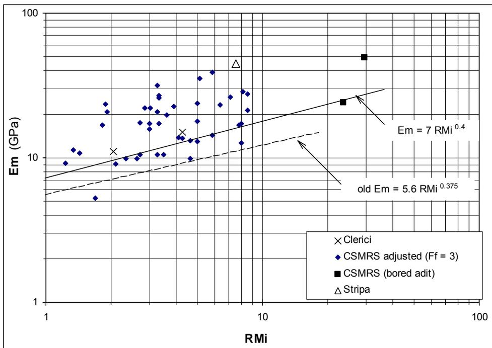
Figure 11: Connection between  $RM_i$  and deformation modulus ( $E_m$ ). The CSMRS (blasted) results have been adjusted with a field factor  $F_f = 3$ .
