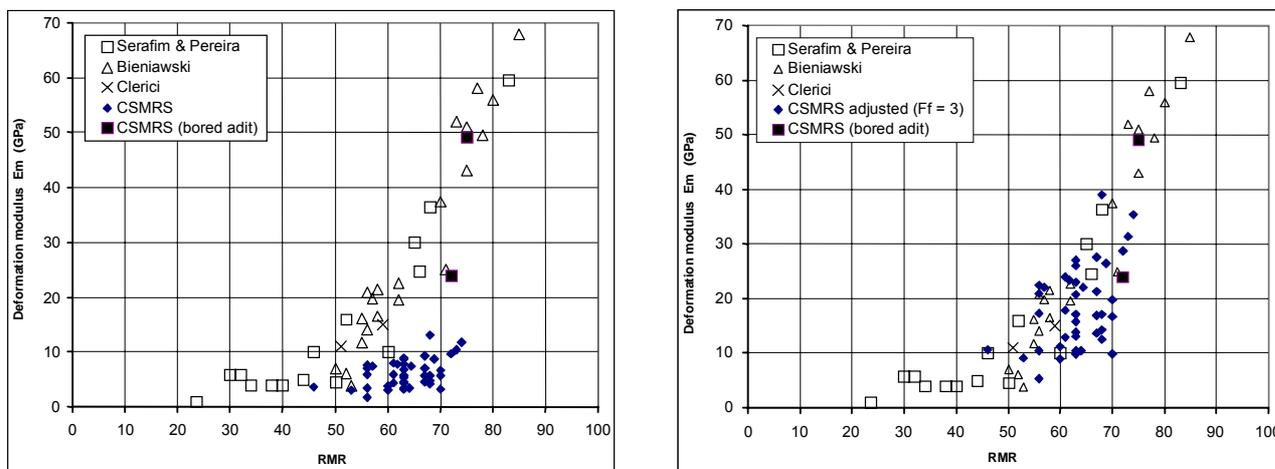
Figure 8: Left: CSMRS deformation measurements compared to those of Bieniawski, of Serafim and Pereira and of Clerici. The two measurements conducted in the “bored” adit are within those of Bieniawski etc. Right: The CSMRS measurements have been adjusted for blast damage with  $F_f = 3$
