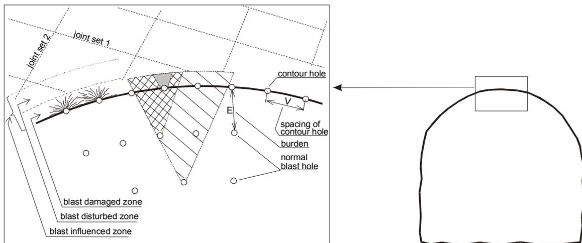
Figure 5: Damage zones from different hole rows (based on Holmberg et al., 1979). Reduced charges in the contour holes create a smaller damage zone than the normal blast holes. Also the burden and the charges in the holes nearest to the contour holes are important features in cautious blasting to reduce blast damage.
