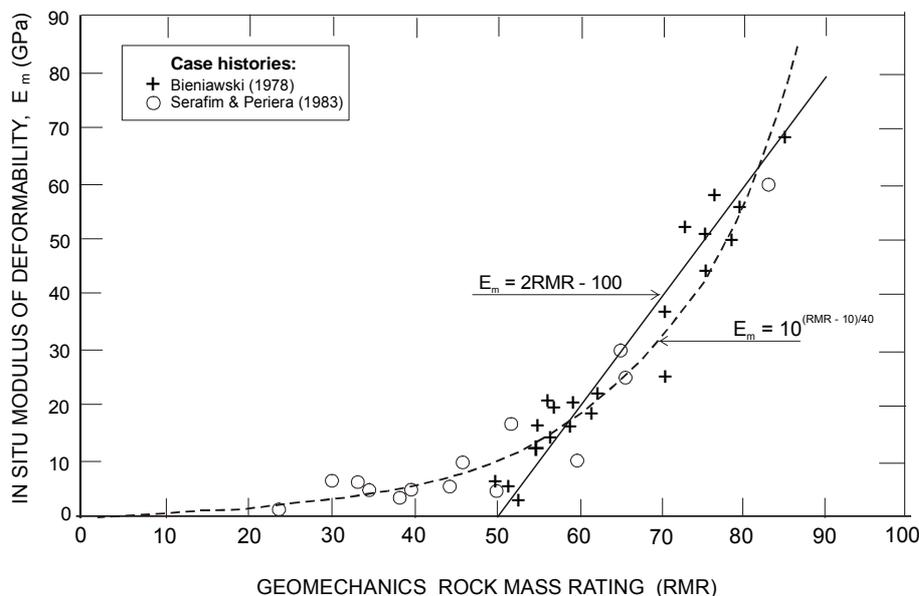
Figure 4: Correlation between the in situ modulus of deformation and the RMR system (from Serafim and Pereira, 1983)
