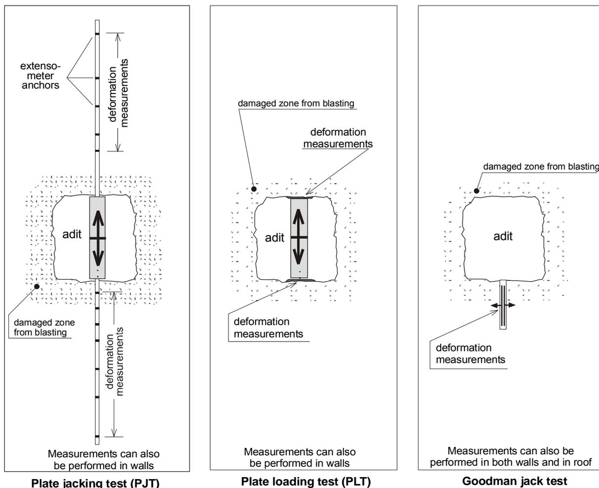
Figure 2: Principles of three main methods for in situ deformation measurement.
