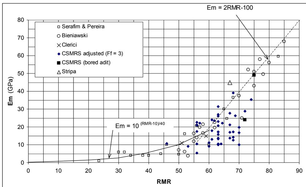
Figure 9: Connection between RMR and deformation modulus ( $E_m$ ). The CSMRS (blasted) results have been adjusted for blast damage with a factor  $F_f = 3$
