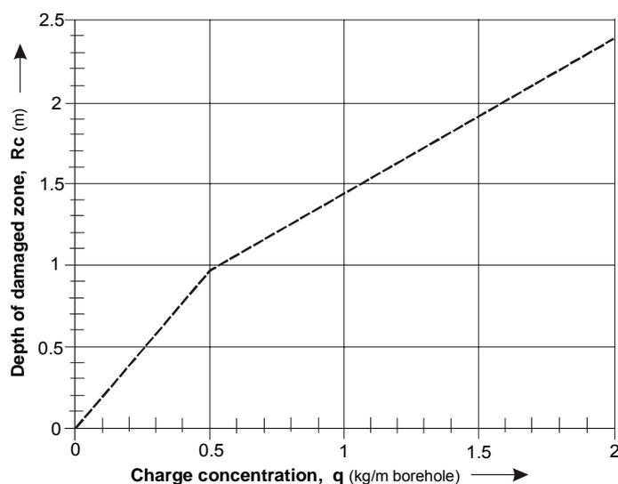
Figure 6: Chart to find the blast damage zone from charge concentration (from Ouchterlony and Olsson, 2000). For test adits where 22 mm glynite or similar explosive has been used,  $q = 0.4$  kg/m and hence the damage zone  $R_c = 0.8$  m
