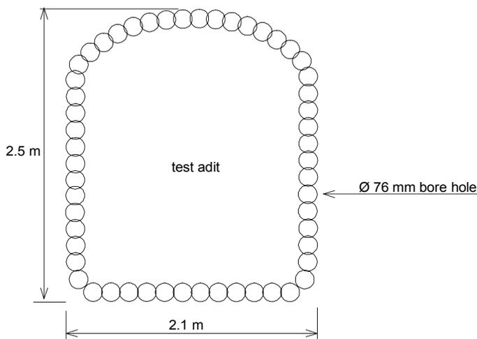
Figure 7: The procedure for excavating the bored test adit at Lakhwar dam project
